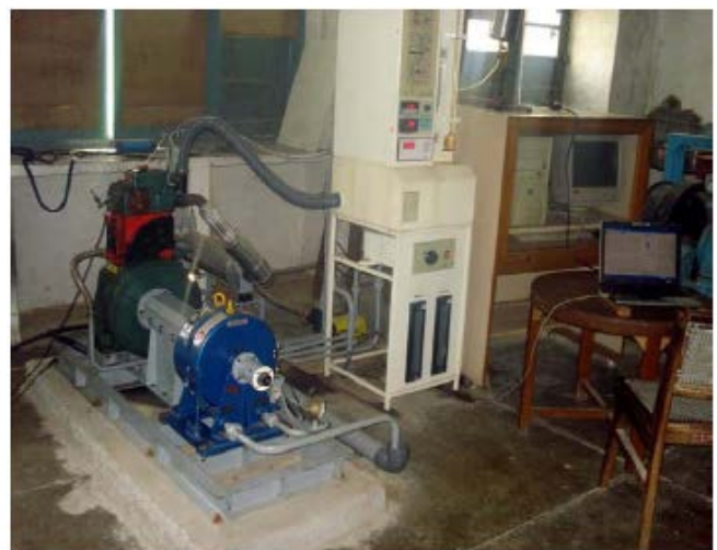
Plate. 1 Variable compression ratio (VCR) engine test setup
